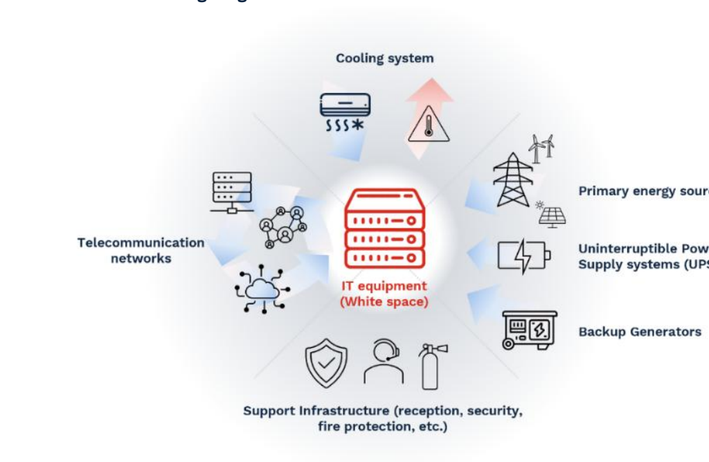
Figure 1 – Core infrastructure elements in a data center and their relationship with IT equipment (white space). Source: Bip analysis.
